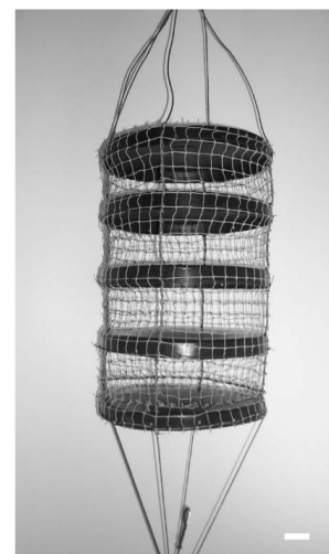
Figure 2 (Right) Design of a lantern for aquaculture of marine sponges as designed for the study of (Kelly et al., 2004). Diameter of the plastic base trays is 61 with 5-cm-high sides facing downwards to provide shadow for the layer below. The sponges are protected against predators by a nylon net with 40mm 2 mesh size. (Scale = 10cm)
